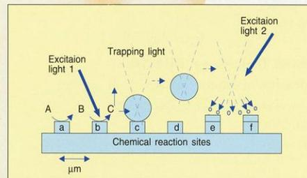
A schematic diagram of Microphotoconversion system which is partially realized
